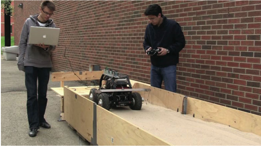
Fig. 21.2 Testing of soil parameter estimation using Quadrover in dry sand
