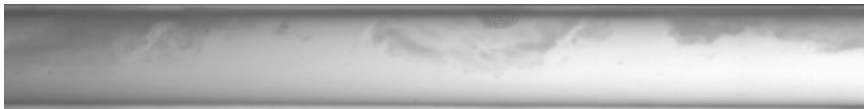
Fig. 20.4 High-speed camera visualization of pneumatic conveying of alumina in bypass pipe (Flow direction is from left to right). a Bypass flutes position. b Immature dune flow- case 7. c Slug flow- case 9
