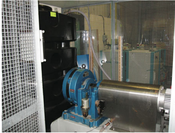
Fig. 2.7 Dynamometer for load testing gearbox
