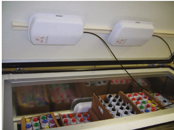
Fig. 48.4 RFID antenna locations for smart freezer solution
