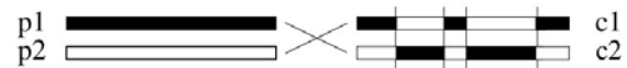
Figure 3. Multi-point crossover between parents p1 and p2 , resulting in children c1 and c2
