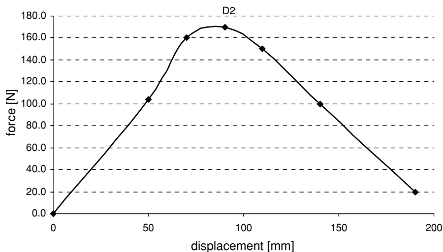
Figure 3. Typical force–displacement curve for a pullout test on vetiver grass (sample D2). The uprooting force increased with displacement to its peak value and then started to decrease due to root slippage or breakage.
