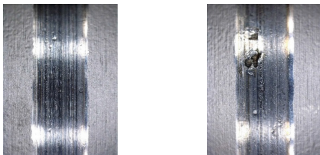
Micropitting, steel 14 220, 11 \times 10^6 cycles Macropitting, steel 14 220, 202 \times 10^6 cycles
