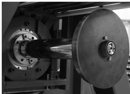
Fig. 1 Photo of extended spindle of CNC machine with weights and laser beam battery source
