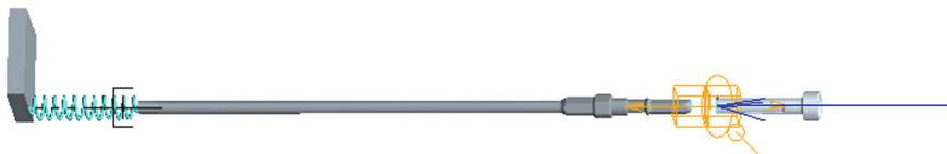
Fig. 2 Assembly for the impact analysis, Creo mechanism
