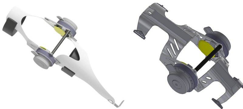
Fig. 4 Robotic orthosis composite and metallic variant
