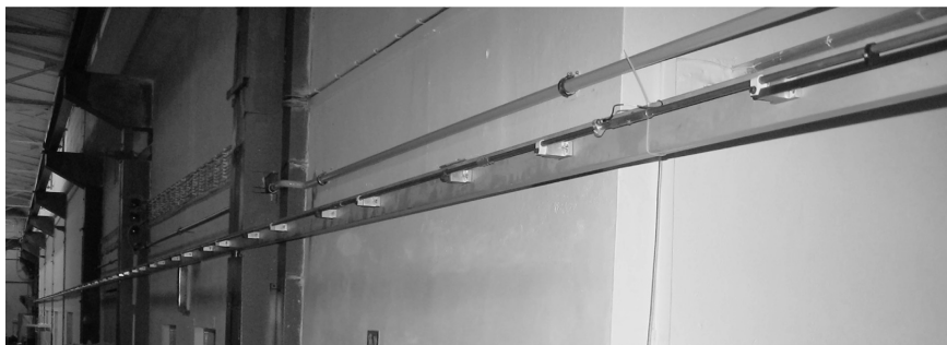
Fig. 4 Measuring set-up with long traversing rod
