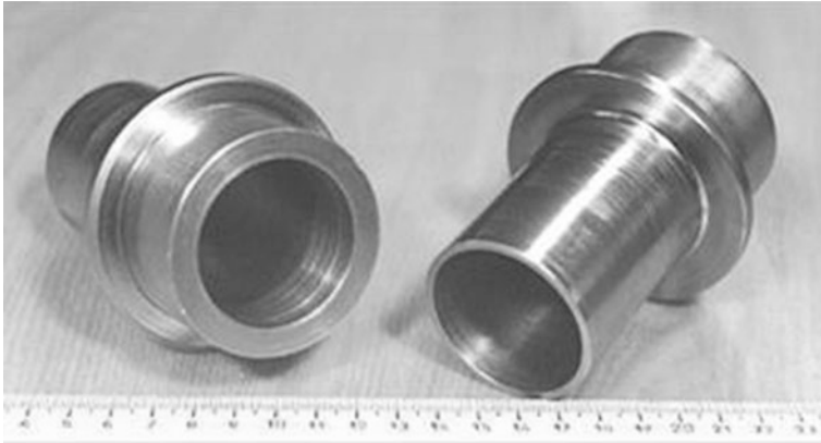
Fig. 1.4 Rotary forged parts from tube-blanks
