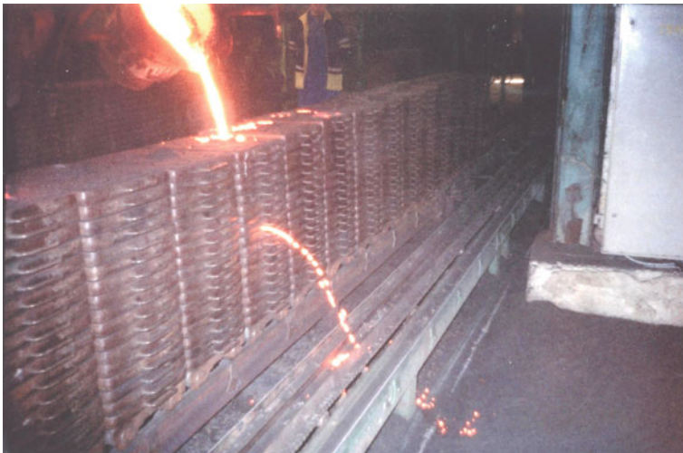
Fig. 9.1 Destruction of a filling form at the overestimated provision of a ladle with metal
