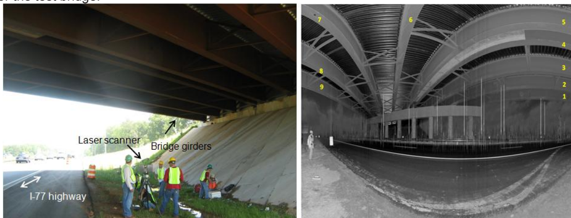
Fig.4 LiDAR scan testing and image of the test bridge
