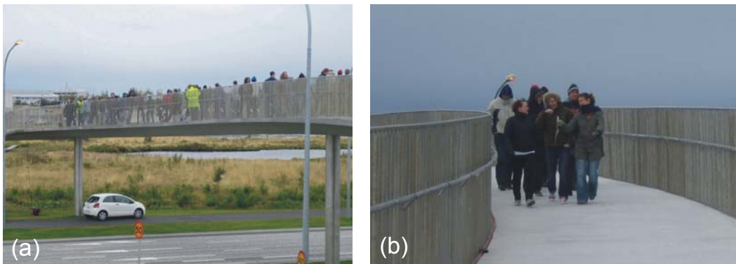
Figure 6: (a) Test 25: all participants walking over Span 2 in circular manner. (b) Test 16: eight people walking across the bridge.
