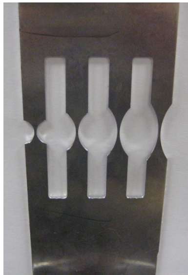
Figure 1: A prototype fatigue sensing element used for Proof-of-Concept
