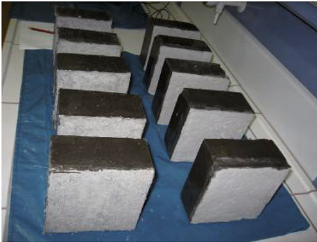
Fig. 4.8 Specimens after 28 freeze-thaw cycles, left side: SHCC specimens, right side: reference mortar specimens.
