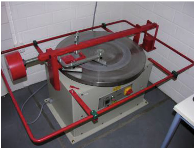
Fig. 2.20 Grinding disc for abrasion testing according to the German standard (E DIN 52108 2006).
