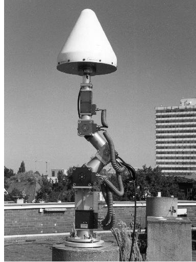
Figure 7.58. Robot for the absolute field calibration of GPS antennas
