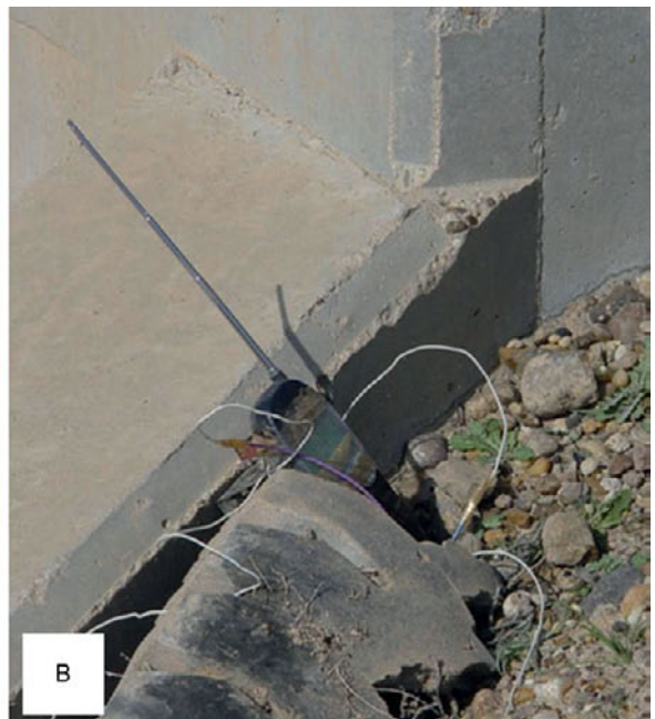
Figure 10.24 (A) Unexploded ordnance is readily available in combat zones from multiple previous conflicts and is commonly used in IEDs. (B) As commonly seen, a rudimentary cellular phone is used as part of a remote triggering mechanism.
