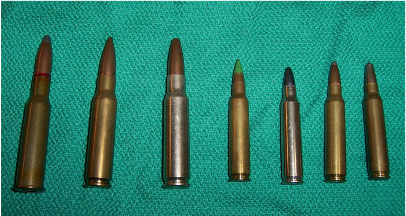
Figure 10.9 Examples of high-velocity bullets typically used in military and hunting weapons. Note the jacketing used to prevent lead stripping as the bullet travels down the barrel.
