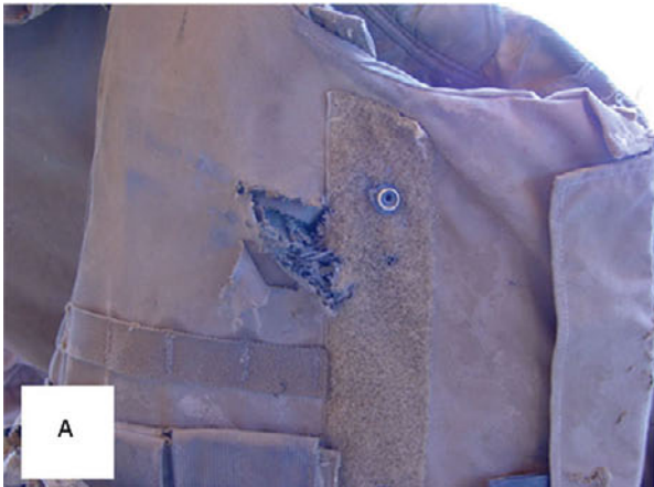
Figure 10.14 (A) Ballistic vests are made from multiple layers of strong woven fibers. The layers are designed to “catch” a bullet, thereby deforming it, and dissipating its energy to a larger area of the vest. Ceramic plates are added to ballistic vests to afford protection against high-velocity rounds. (B) Blunt injuries can occur beneath the vest as the body absorbs the remaining energy from the round.
