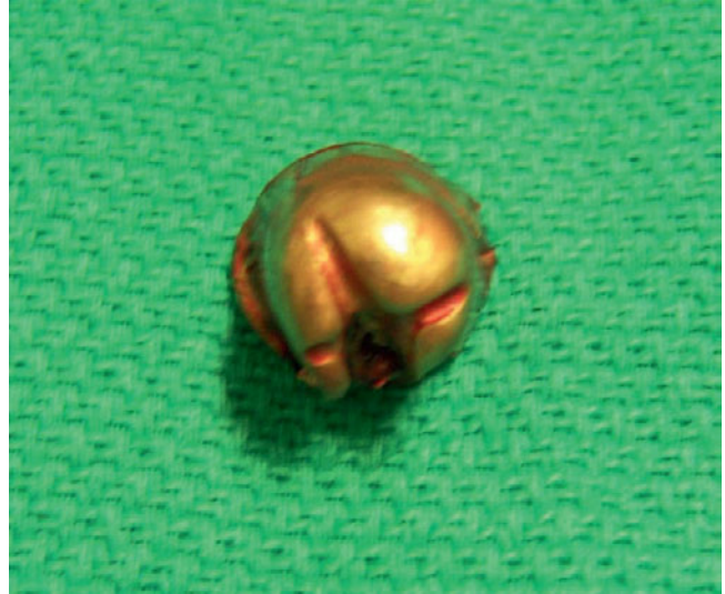
Figure 10.3 Bullet scoring promotes fragmentation on impact and increased tissue damage.
