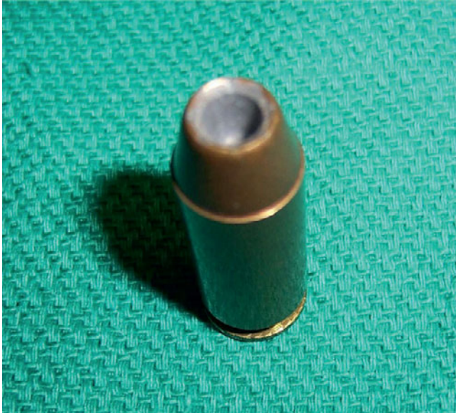
Figure 10.1 Hollow-point bullets are designed to expand on impact and transfer kinetic energy to the target.
