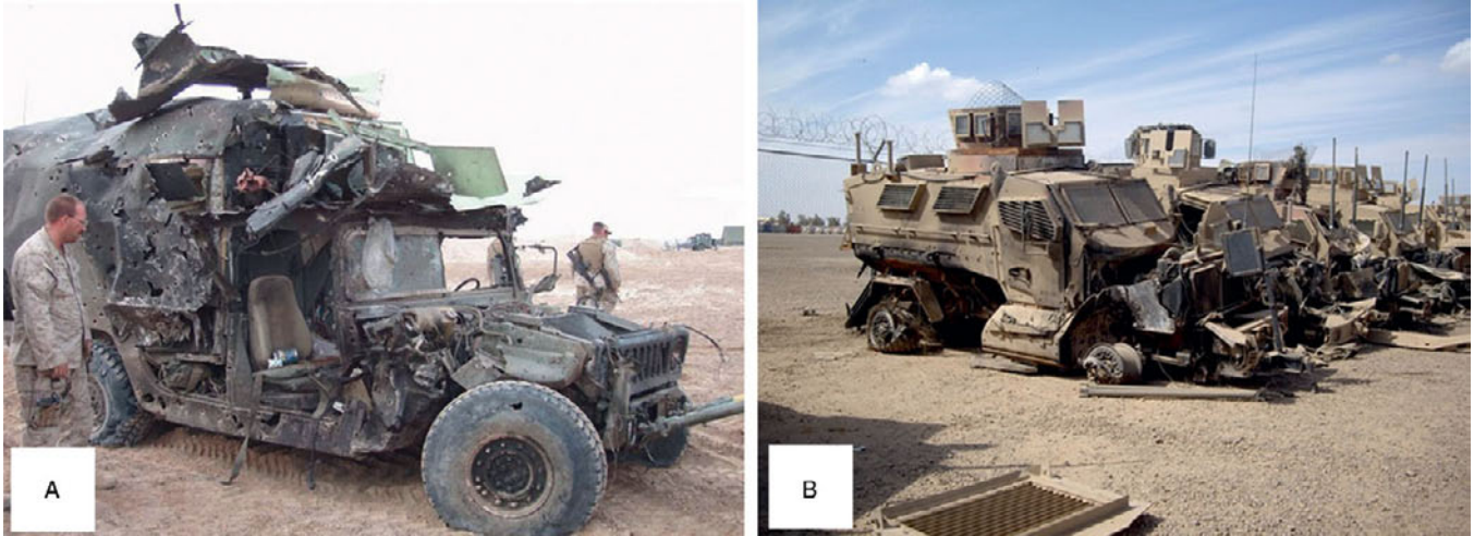
Figure 10.25 Improvised explosive device (IED) injuries. (A) Occupants of unarmored vehicles, such as this military ambulance, are essentially defenseless against the effects of a roadside IED. (B) In “Mine Resistant Ambush Protected” (MRAP) vehicles the passenger compartments remain relatively intact due to up-armorings and the blast-deflecting V-shaped undercarriage. Significant injuries from blunt trauma can still occur due to violent displacement of the occupants within the passenger compartments.
