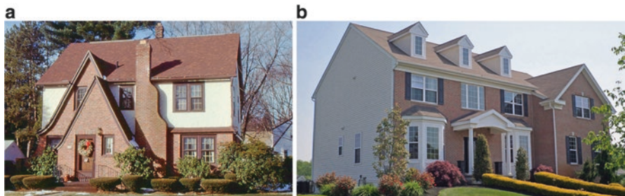
Fig. 7.13 (a) Veneers that appear integral to a design are more appropriate than those that look merely applied. (b) Masonry used on the facade of a house looks bad when it appears to be pasted only onto the full height of the front facade only
