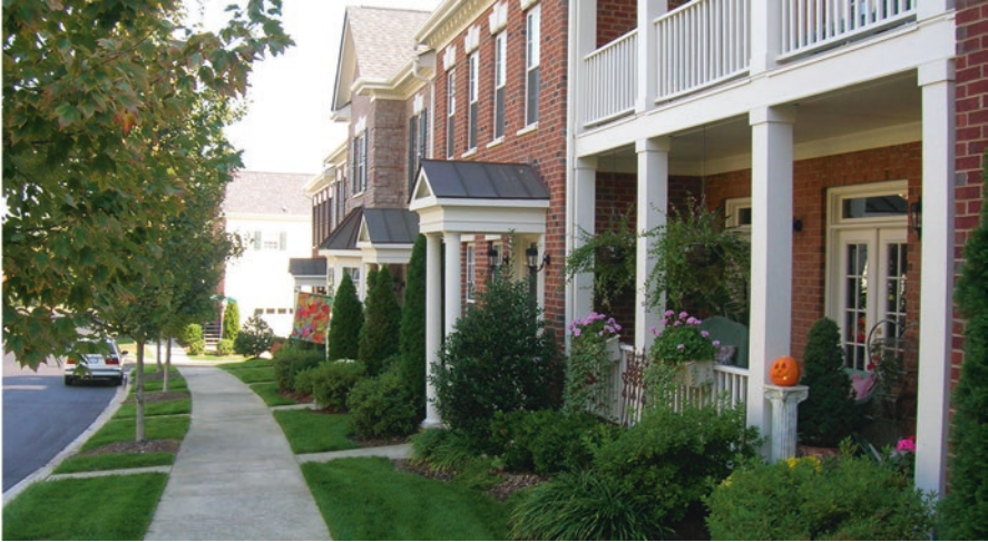
Fig. 8.3 Attached houses generally need to be set apart from one another. A clearly individual front door, separated from the adjacent houses, is optimal. Changes in window and door patterns, as well as material and color changes, will also help differentiate each house from its neighbor
