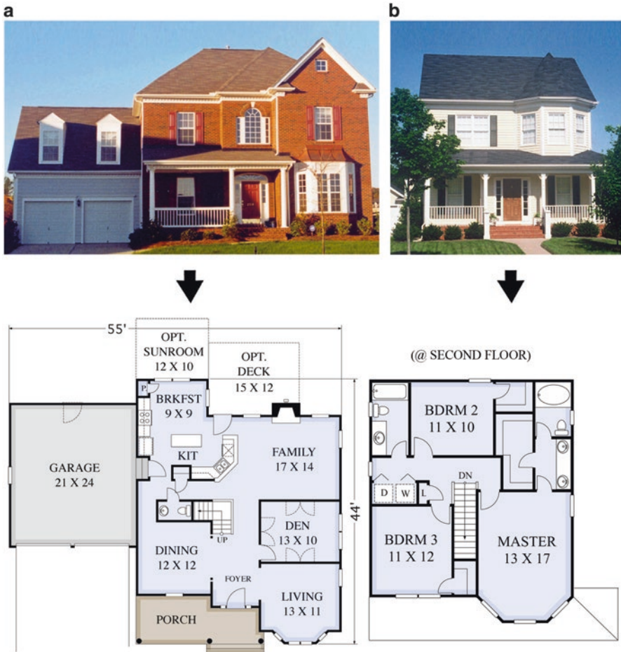
Fig. 6.12 (a) Bay windows are a traditionally popular design feature generally found in formal living or dining rooms. (b) The idea behind window bays can be extended to projecting walls of entire rooms, such as in a second floor master suite or bedroom
