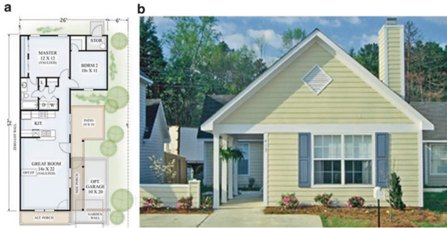
Fig. 5.15 At Breckenridge , these very affordable houses were primarily 14 ft wide, reminiscent of Southern “shotgun” houses. (a) The narrow spans helped to maximize penetration of light into rooms. (b) Such a plan allows more rooms to view the private outdoor courtyard in the sideyard area
