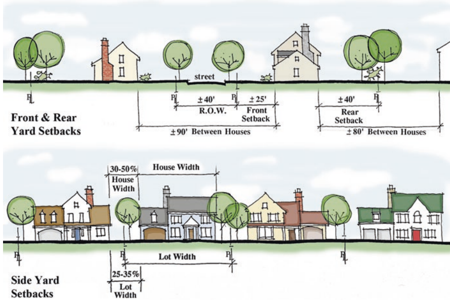
Fig. 4.2 For houses on conventional lots, the front, rear, and side yards should all be proportional to the lot and house dimensions
