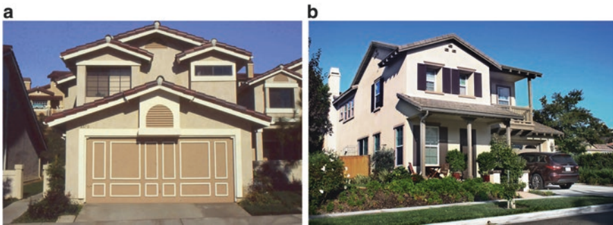
Fig. 12 (a) Lots were too small in many Sunbelt markets, resulting in houses with narrow frontages dominated by garage doors. (b) These “wide/shallow” lot houses at Bressi Ranch built by Lennar outside of San Diego recess the garage and include front porches facing the street. (Photo (b) courtesy Tom Voss)
