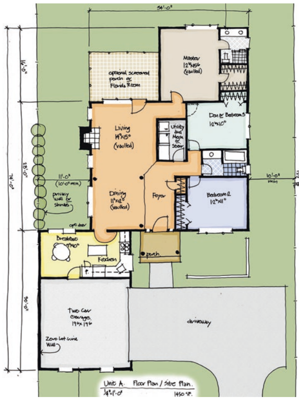
Fig. 4.25 This design with a turned garage orients the driveway and garage doors away from the street. This concept is popular for narrow lots, but parked cars can potentially block the view of the entry area
