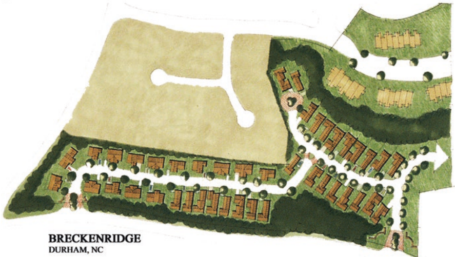
Fig. 3.9 (a) Excessively wide streets destroy human scale in residential neighborhoods, increase impervious surface coverage on site, encourage speeding cars, and waste space. (b) At a neighborhood in Durham, NC, narrower 24-foot-wide private streets were approved to reduce development costs
