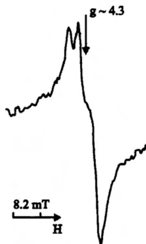
Figure 2-8. The EPR spectrum of human blood plasma. The registration conditions: temperature - 77^\circ\text{K} , SHF power - 5 mW, magnetic field scanning velocity - 10 mT/min, HF modulation - 0.5 mT, the time constant - 0.3 sec.
