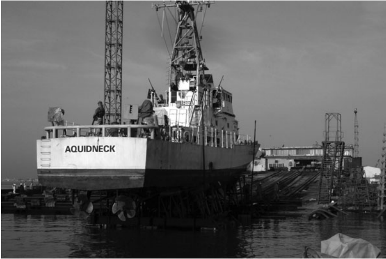
Figure 1-5. Marine railway. U.S. Coast Guard photo by PA2 Kyle Niemi.
