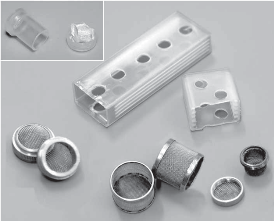
Fig. 6. Small holders used to protect small specimens during the critical point drying procedure. Inset, top left corner, shows holder fashioned from polypropylene embedding mold used in transmission electron microscopy. Large, rectangular container is a microscope slide mailer that has been modified to hold slides and cover slips. The three sets of stainless-steel mesh holders are commercially available.
