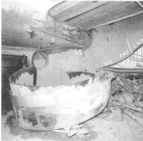
Figure 1.6 Burst high pressure preheater and devastated plant room: After Schaden Spiegel 1/82
