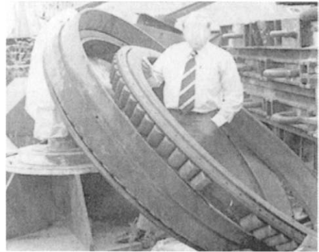
Figure 7.10 The failed main bearing with the works supervisor (approximately 1.7 m tall) indicating the scale. The bearing is situated in the vicinity of the "muck ring" indicated in Figure 7.9.
