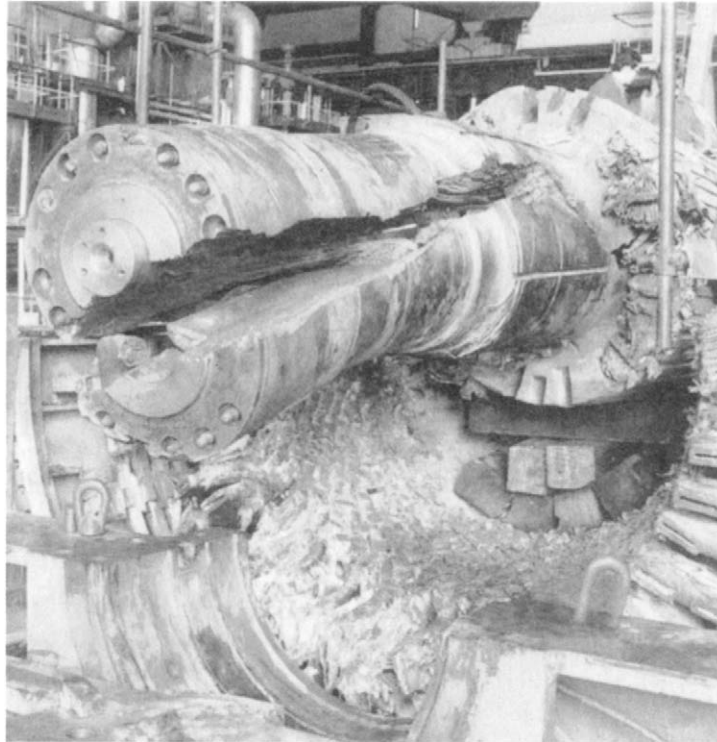
Figure 1.5 Failure of the main shaft of a 600 MW turbogenerator set: After Schaden Spiegel 1/82
