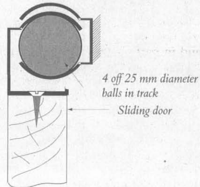
Figure 2.61 Schematic section through sliding door track.
