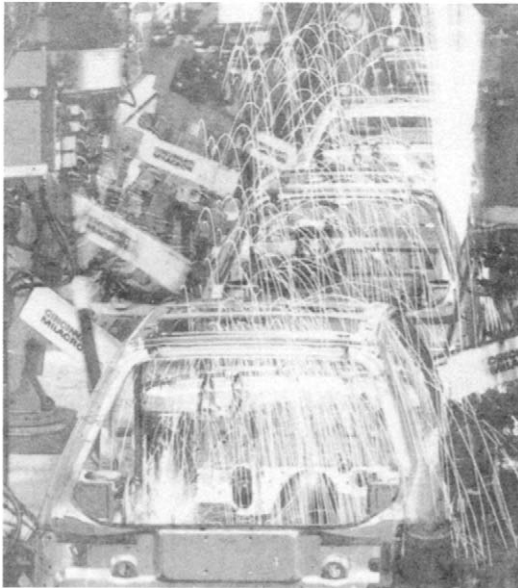
Figure 4.41 Robotic welding in automotive manufacture
