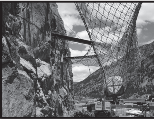
Photograph 5. Broken Post Resulting from Test I. (Per ETAG 27 this could be considered a Category A test since it stopped the rock and the residual height would be greater than 50 percent).
