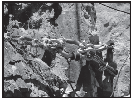
Photograph 4. Center of Photograph Shows Link Cell for Measuring Tensile Loads in Wire Ropes.
