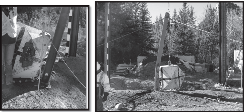
Photograph 22. Results of 217.5 kJ test for G series test.
