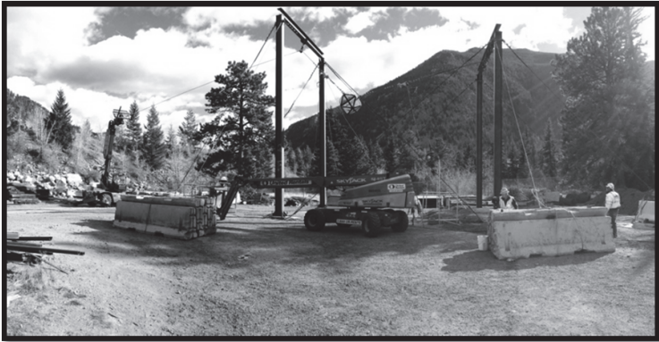
Photograph 8. Side view of the test site setup. Rock is released and swings to right side of photograph.
