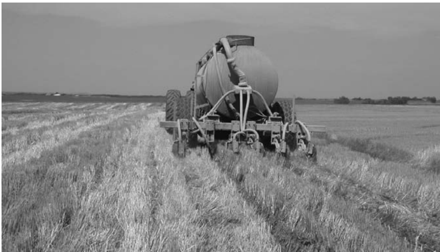
FIGURE 3.5 Swine manure injection with sweep blades 8–10 inches (20–25 cm) below the soil surface.
