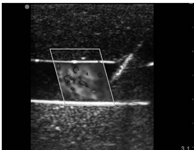
Figure 20.78. Ultrasound image showing turbulence within a phantom vessel highlighted by color Doppler.
