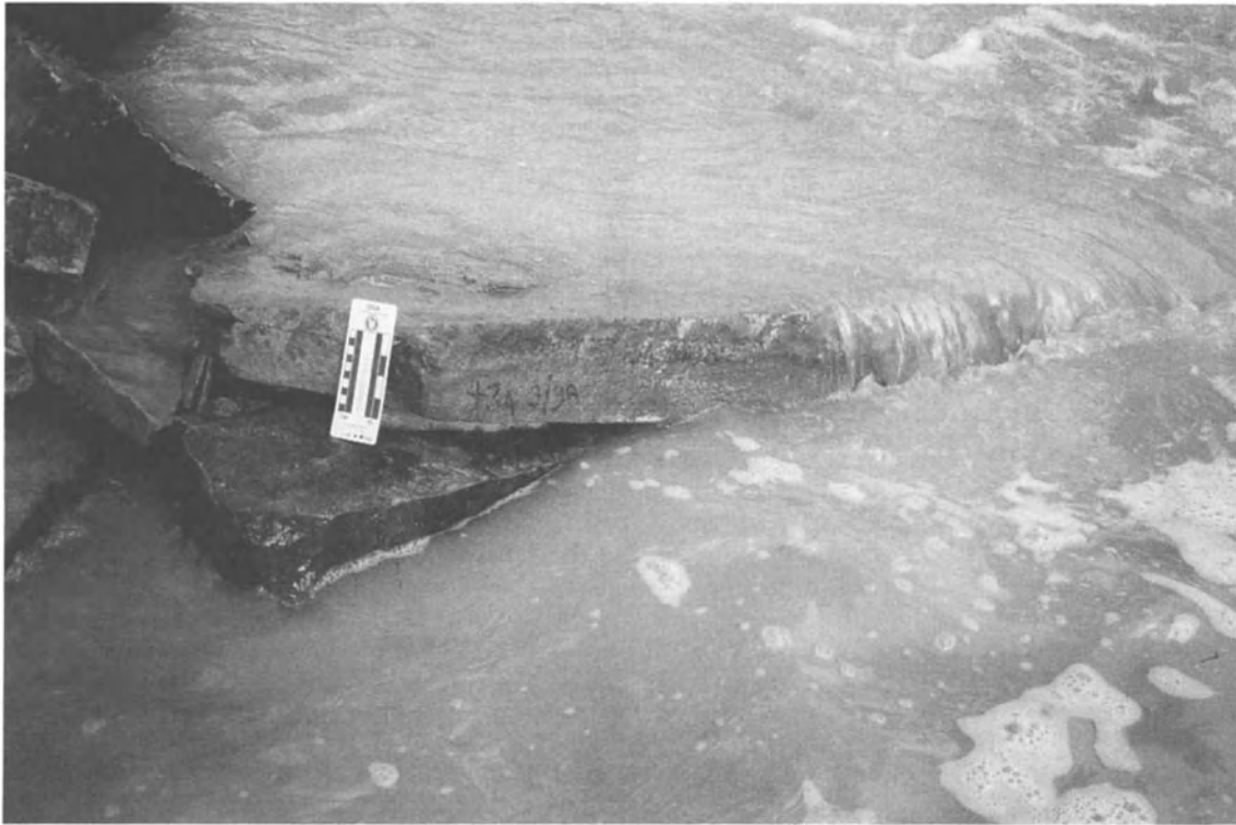
Figure 3. Clast marked with indelible marker moved from 25 meters up river and deposited in imbricate position at the channel margin. Looking upstream the clast is 1.8 metres long (across picture and transverse to flow), 55 cm wide and about 15 to 20 cm thick.
