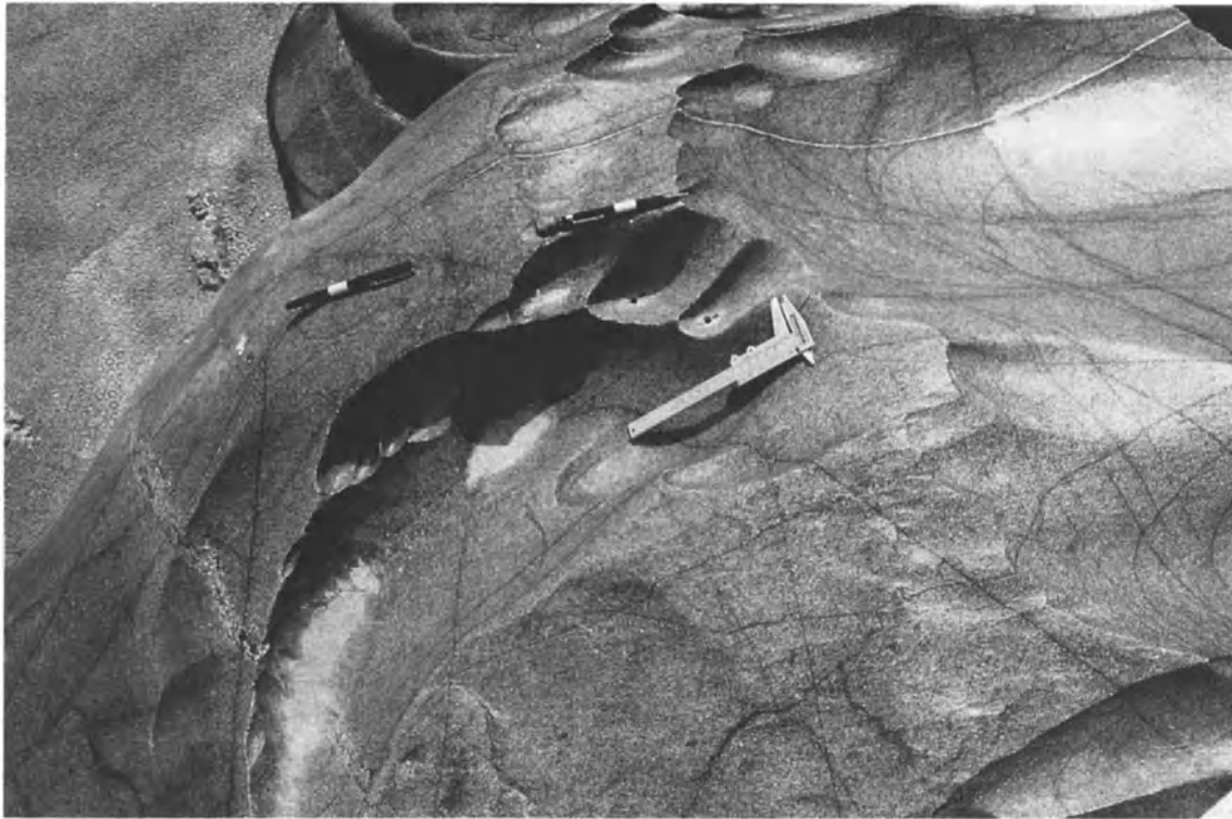
Figure 11. Example of drill hole placement (Site C, Figure 10). Flow is left to right, and reaches ~10 m depth during maximum flows. Note hole placement on smooth upstream faces (left of leftmost pen), and within flutes (between pencil and vernier caliper).
