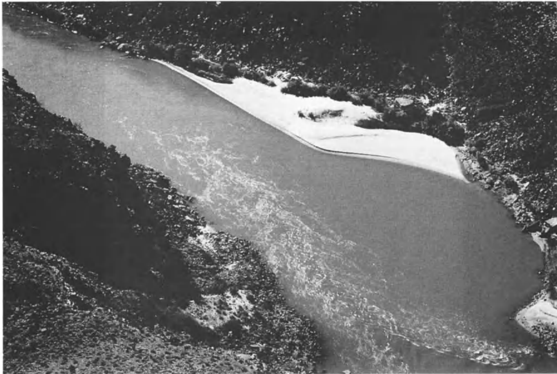
Figure 11. Oblique aerial photograph (taken in October 1991) showing incised channel, coarse debris-channel constriction, and associated fine-grained sand deposits. Flow is from the bottom to top of the photograph. Location is in the Grand Canyon, approximately 370 km downstream from Glen Canyon Dam.
