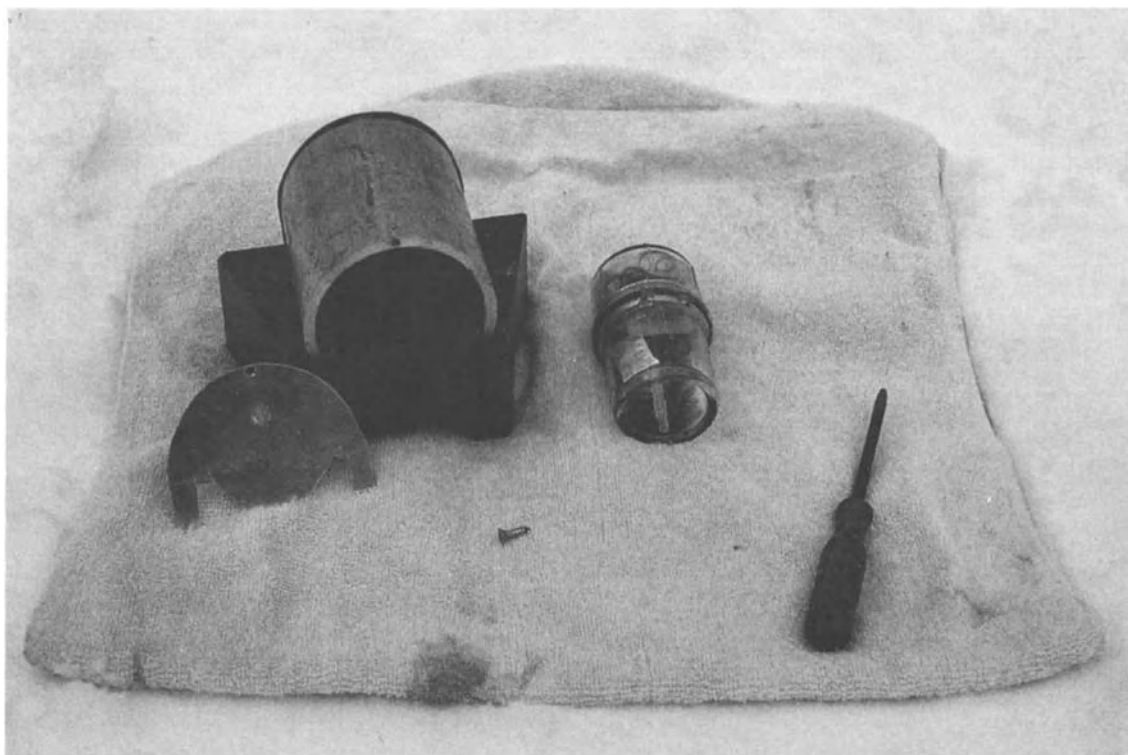
Figure 6. The waterproof bottle contains a 32K Stowaway logger and stand-alone pressure transducer for recording very short term changes in water level (see Figure 8). The pale tube just visible at the bottom of the bottle transmits water pressure through an oil-filled tube to the transducer. The housing is an aluminum pipe screwed to an 8 kg lead footing. Sampling time of 40 seconds optimizes the ability to capture short term water surface fluctuations, and the observer's ability to retrieve the gauge on the falling stage before it overwrites the record.
