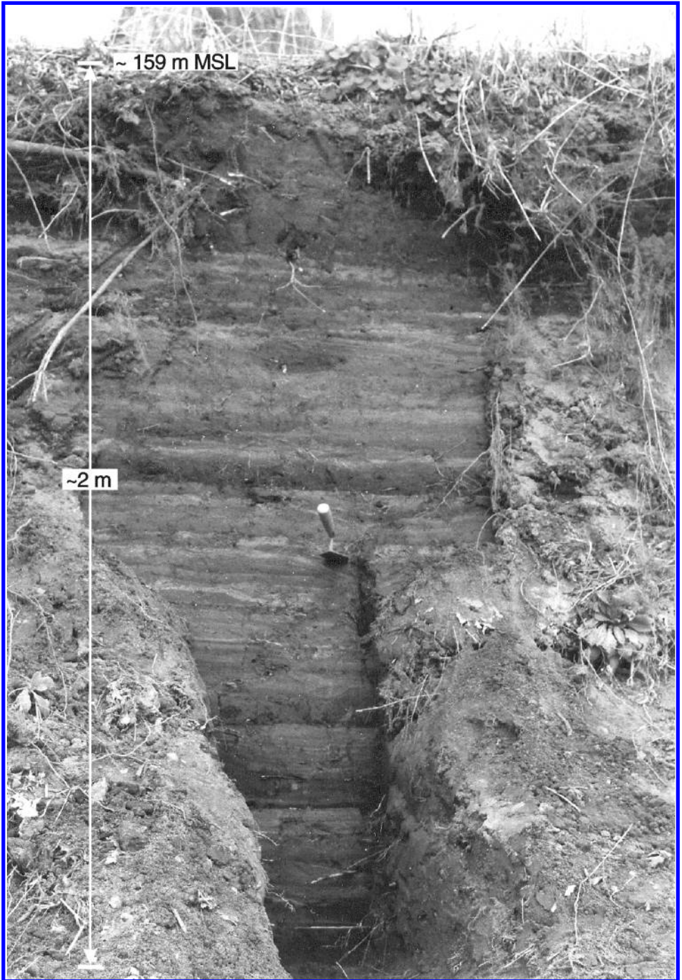
Figure 6. Terrace remnant constructed by slackwater in the pool behind a crib dam at Nanticoke, Pennsylvania for the North Branch Canal.
