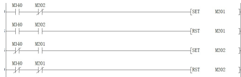
b) Corresponding ladder diagram
