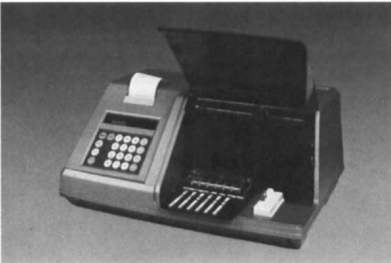
Fig. 7. Cobas Ready system, open front door.
