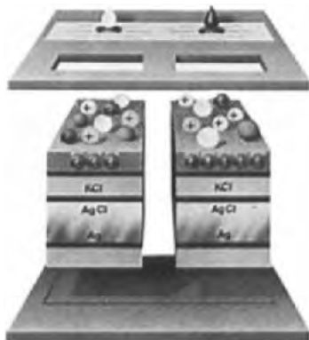
Fig. 14. Representation of a slide for the assay of electrolytes by the Ektachem system.
