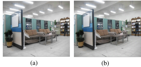
Fig. 11. Comparison between original and corresponding recovered images. Average PSNR of recovered area is 30.37. (a) Original image. (b) Recovered image.
