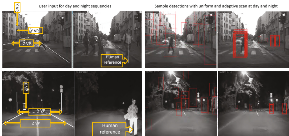
Fig. 5. Left: User input for vanishing point estimation (left) and human reference object (right). Right: Sample detections by using uniform(left) and adaptive(right) scans.
