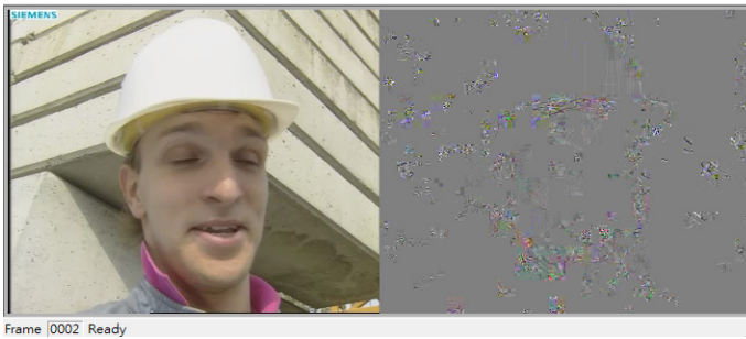
Fig. 2. The left decoded picture is coded by our proposed algorithm, and the right residual picture is the difference between the left picture and the coded picture by JM at QP = 22. The differences are 10 times magnified.
