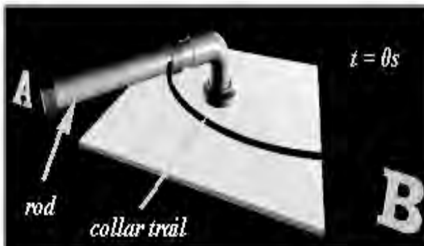
Figure 9. Linear motion of the rod and collar rotating along y-axis ( t = 0s )
