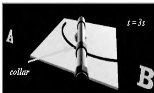
Figure 10. Linear motion of the rod and collar rotating along y-axis ( t = 3s )
