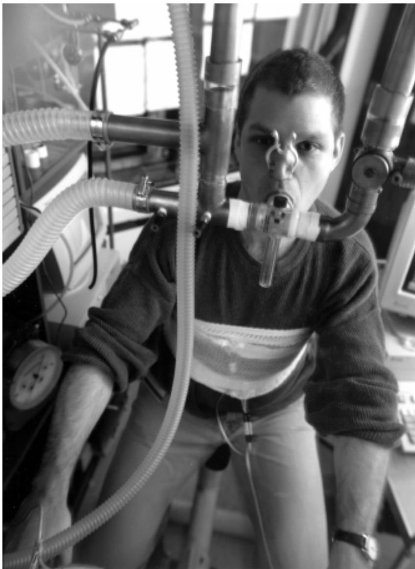
FIGURE 2-8 Exercising volunteer being exposed to ultrafine particles and monitored for health response. SOURCE: HEI 2000. Reprinted with permission; copyright 2000, Health Effects Institute.
