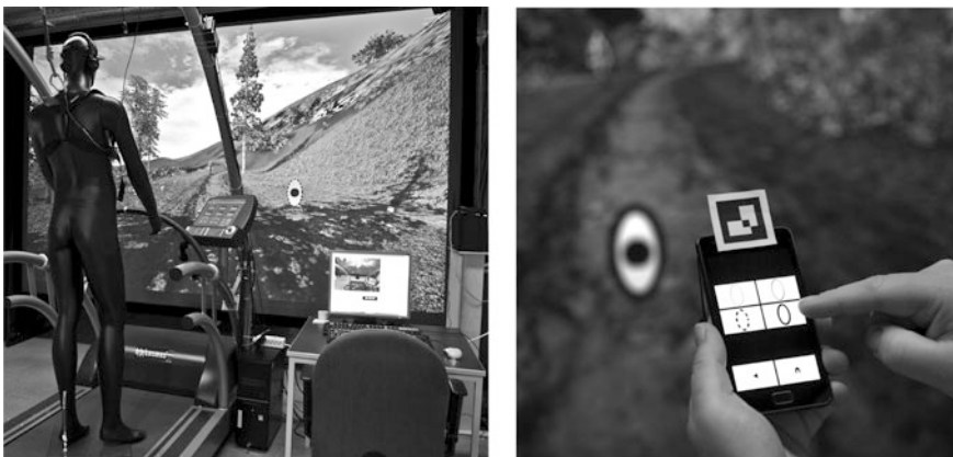
Fig. 1 Apparatus of the study, including powerwall and treadmill ( left ) and interaction device ( right )
