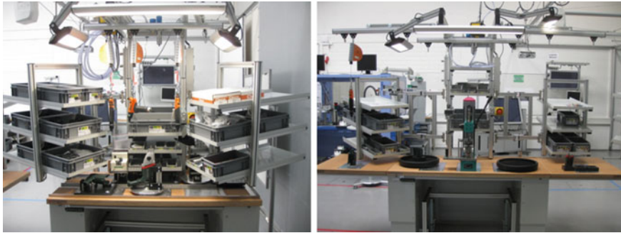
Fig. 1 Adaptable assembly workstation (on the left single- and on the right triple- workplace)
