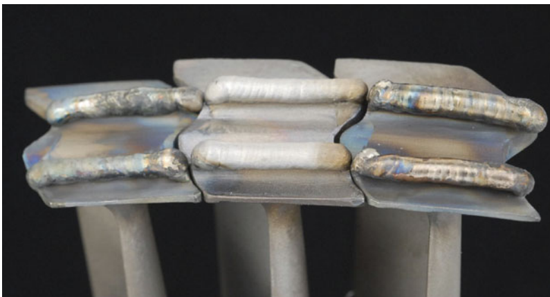
Fig. 4 Photograph of compressor blades after manual weld deposition
