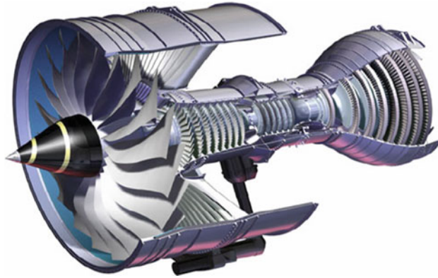
Fig. 1 Cross sectional rendering of Rolls-Royce Trent1000 turbofan engine detailing the removable compressor blades in the central section
