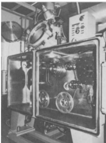
Fig. 2 Continuous liquid quenching apparatus. 12
