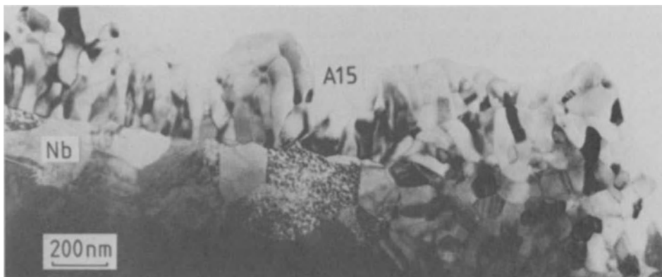
Fig.5 TEM micrograph of Wah Chang MJR composite M88 after a reaction heat-treatment at 650°C for 49 hours.
