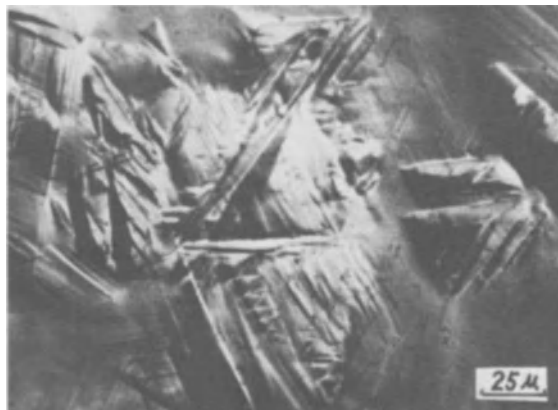
Fig. 2. Microstructure of the Fe-14Mn-0.4C alloy revealed by Nomarski interference contrast metallography.
