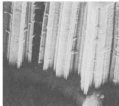
b) Detail of the filaments (defects are undissolved matrix). Filament diameter = .12 micron.
