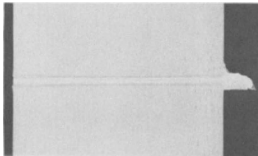
Photo 1. The macroscopic cross-sectional view of the electron-beam-welded 22Mn steel (70 mm thick).
