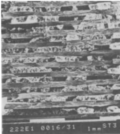
Fig. 8. SEM fractograph of the G/E bend specimen at 190 K.
