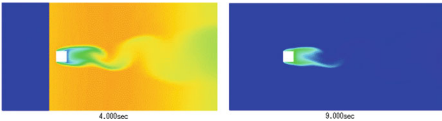
Fig. 7 The computed distribution of smoke concentration of the case of isotropic diffusion K = 1.0 \text{ cm}^2/\text{s} at t = 4.0\text{s} and 9.0\text{s} .
