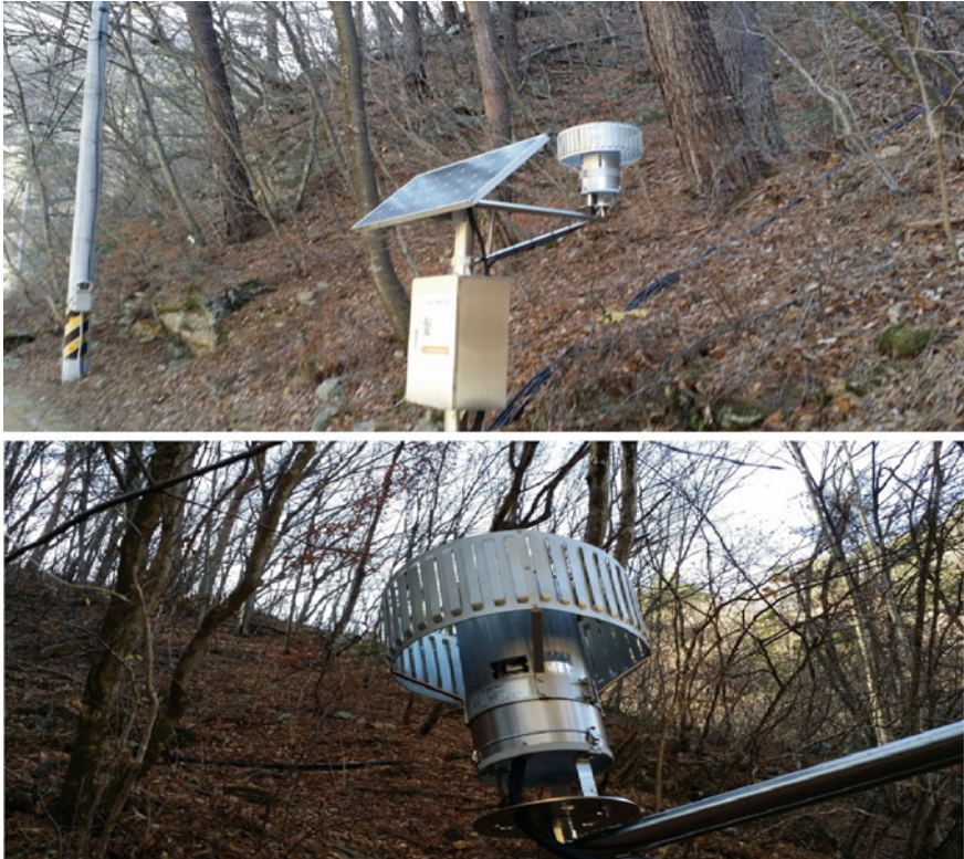
Fig. 4.32 Measuring system of precipitation and snowfall with its protector, and a solar panel for power supply, Seoraksan National Park, Korea
