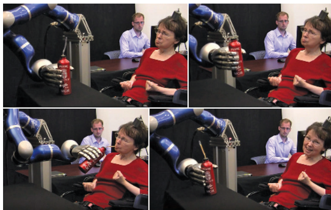
FIGURE 7.7 Recordings from the brain control a robotic arm After a stroke in this woman's midbrain cut off connections from her cortex to the spinal cord, she lost all control of her arm and leg muscles. A neural decoder connected cells in her motor primary motor cortex to a robotic arm, enabling her to pick up a coffee cup, drink from it, and put it back. Source: From L. R. Hochberg, D. Bacher, B. Jarosiewicz, N. Y. Masse, J. D. Simeral, J. Vogel, ... J. P. Donoghue (2012). Reach and grasp by people with tetraplegia using aneurally controlled robotic arm. Nature , 485, pp. 372-375
