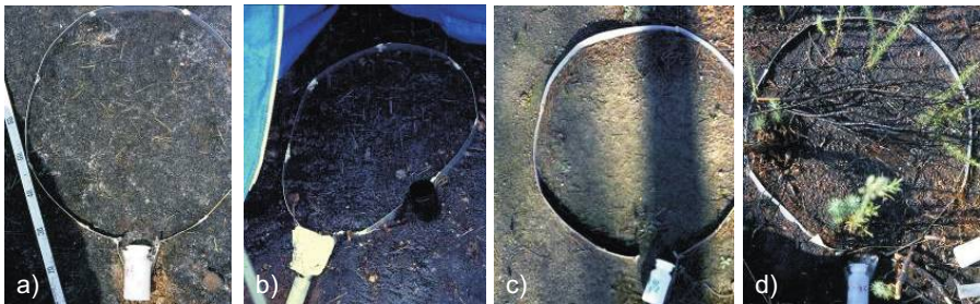
Fig. 2 Rainfall simulation plots from the Pedralba site, Spain. From left to right: a) two days after fire with ash cover; b) during the first simulated rainfall experiment; c) 4 months later with sealed surface; and d) 8 months later with the Ulex parviflorus and Pinus halepensis saplings.
