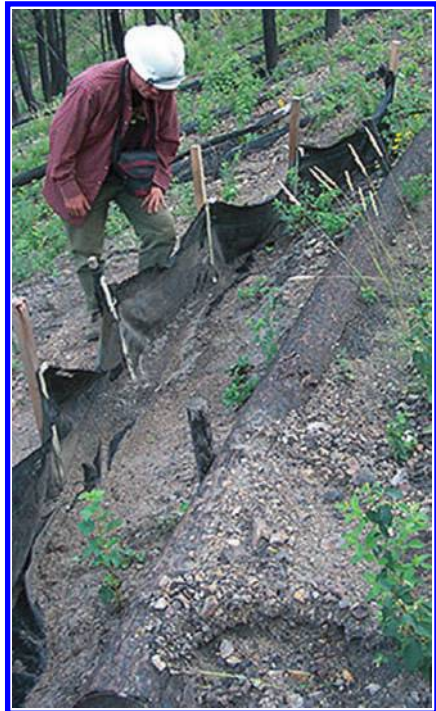
Fig. 5 A hillslope plot research site with a geotextile sediment fence (Robichaud and Brown 2002) one year after installation. This plot is one of 24 plots established after the 2000 Valley Complex Fires in Montana, USA to measure contour-felled log erosion barrier treatment effectiveness.
