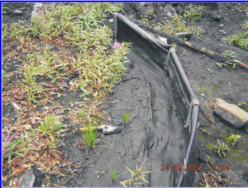
Fig. 1 Soils eroded off a bark mulch experimental plot, that were captured in a silt fence so the mass and water content can be measured, as part of the rehabilitation trial described in the text.
