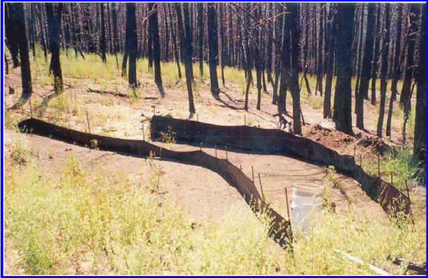
Fig. 6 A hillslope swale research site with a double geotextile fence one year after installation. This is one of 24 swales research sites established after the 2000 Bobcat Fire in Colorado, USA to measure contour-felled log erosion barrier, straw mulch, and seeding treatment effectiveness.
