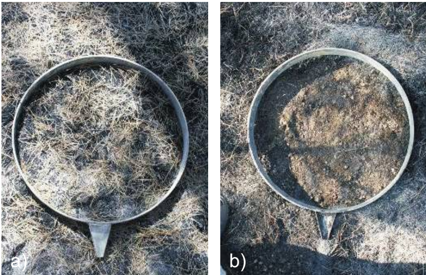
Fig. 4 Naquera study site immediately after fire. a) plot with ash cover; b) bare plot after removal of ash by hand.
