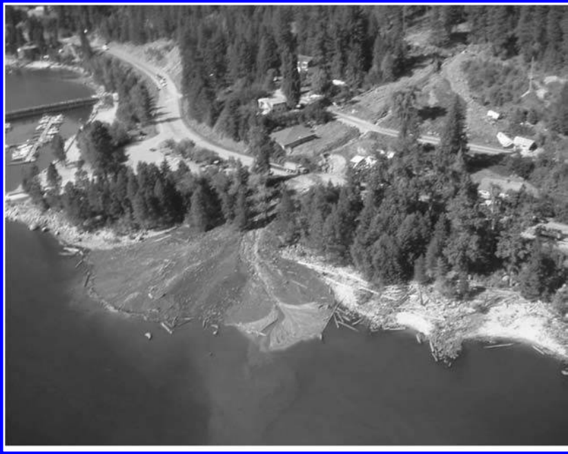
Fig. 3 A debris flow fan that was associated with wildfire in the mountains directly above Kuskanook, British Columbia, Canada. Approximately 60,000 m 3 was deposited on the existing alluvial fan. Photo: Mike Curran, British Columbia Ministry of Forests and Range, Nelson, British Columbia, Canada.
