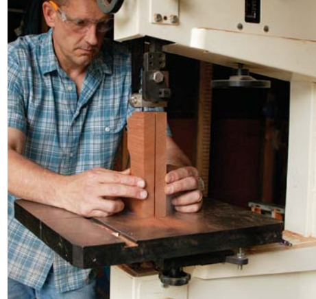
CREATE THE OUTER LAYERS. After kerfing the center of the blank on a tablesaw to guide the bandsaw blade, resaw the outer blank into two halves.
