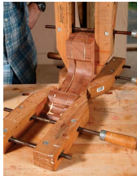
ASSEMBLE THE SANDWICH. The full-width middle piece is flanked on both sides by a half-thickness piece whose profile is slightly prouder in the center. Use a small roller to spread glue on all mating surfaces, then clamp. Make sure all surfaces are aligned and that glue squeeze-out is consistent.
