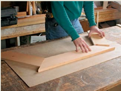
FORM THE CASING BLANK. Segments of stock are cut, then biscuited, glued, and screwed to the layout.
