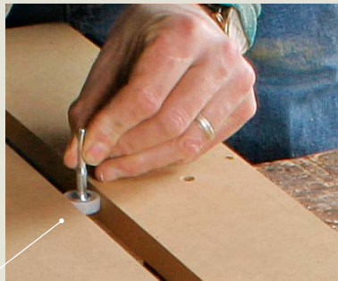
SPACE THE TRACKS. Use the guides for spacing. There should be no slop between the guides and the tracks.
