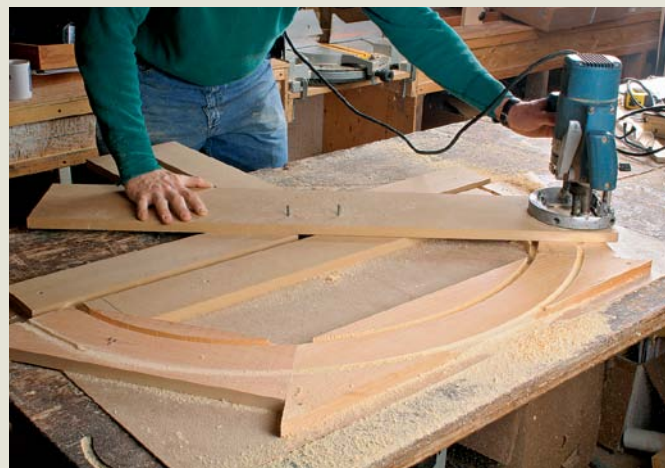
ROUT THE ELLIPTICAL CASING. The rear guide (closest to the author) follows the vertical track; the front follows the horizontal.
