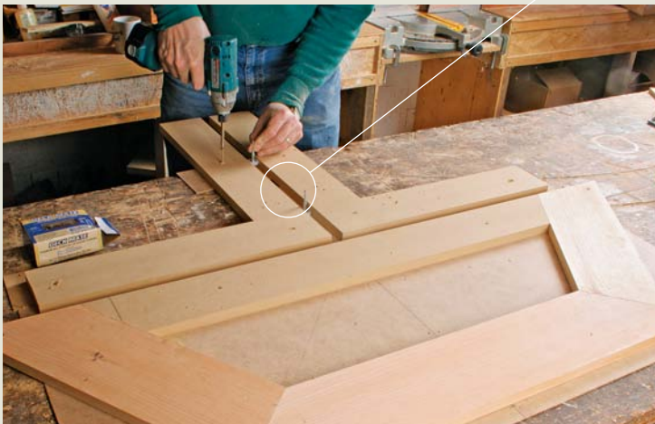
FORM THE TOP OF THE TRAMMEL GUIDE. An additional piece is screwed across the base of the ellipse. The legs of the T center on the minor axis.
