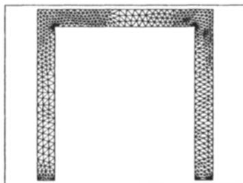
Figure 7. Final mesh optimized with the dissipation error, 661 six-node triangles.
