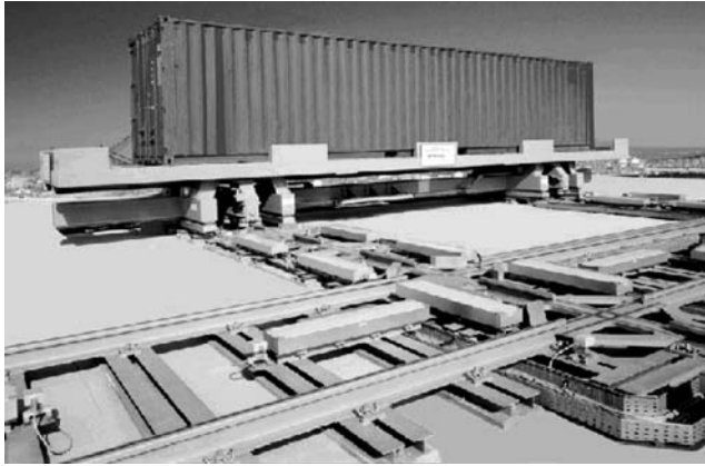
Figure 8.12 LMTT pallet wagon propelled by electromagnetic force
