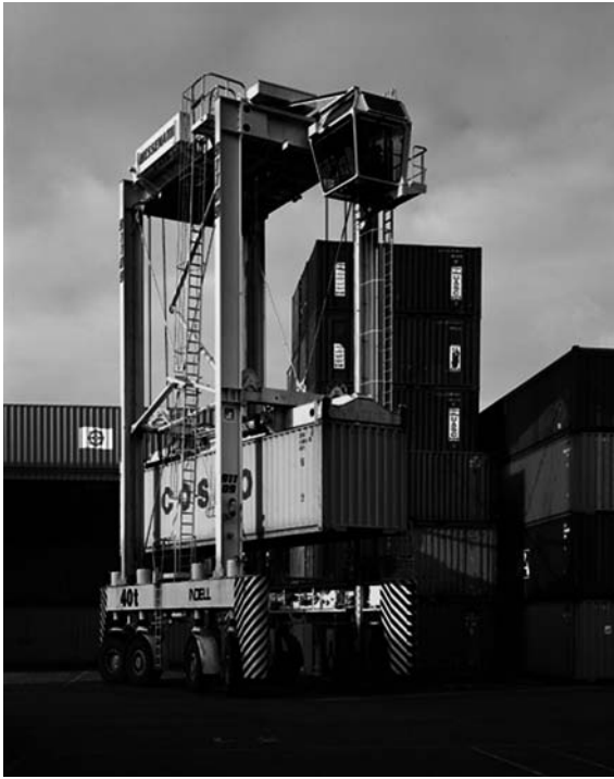
Figure 8.4 Straddle carrier on duty at the container terminal at Hesseantie NV, Antwerp, Belgium
