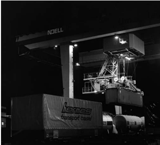
Figure 8.9 Cantilevered rail-mounted gantry crane at the intermodal terminal in BasellWeil, Germany
