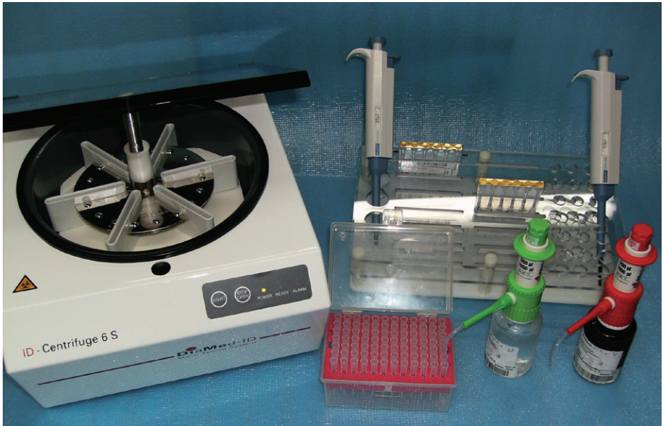
Figure 17.4 Gel typing centrifuge and materials. (Courtesy of Bio-Rad.)
