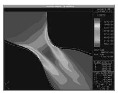
(a) Contour plot of the variation of the shear stress within the flow domain on longitudinal cutting plane; range  $0.00 \, \mathrm{dyn/cm2}$  to  $48.93 \, \mathrm{dyn/cm2}$ .
