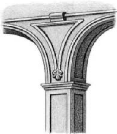
Figure 2.12 The spandrel is the space between the two arches.
