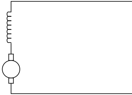
FIGURE 6.93 DC series motor. (From Spellman, F.R. and Drinan, J., Electricity , Technomic Publ., Lancaster, PA, 2001.)
