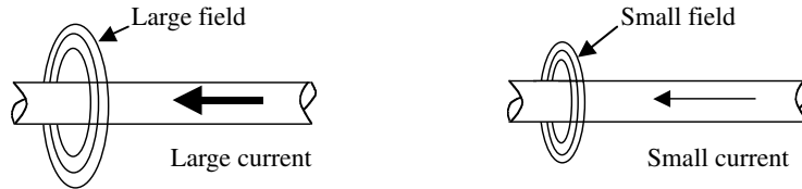
FIGURE 6.63 The strength of the magnetic field around a wire carrying current depends on the amount of current. (From Spellman, F.R. and Drinan, J., Electricity , Technomic Publ., Lancaster, PA, 2001.)
