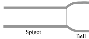
FIGURE 8.10 Bell and spigot ends of clay pipe sections. (From Spellman, F.R. and Drinan, J., Piping and Valves , Technomic Publ., Lancaster, PA, 2001.)
