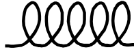
FIGURE 6.78 Schematic symbol for an inductor. (From Spellman, F.R. and Drinan, J., Electricity , Technomic Publ., Lancaster, PA, 2001.)
