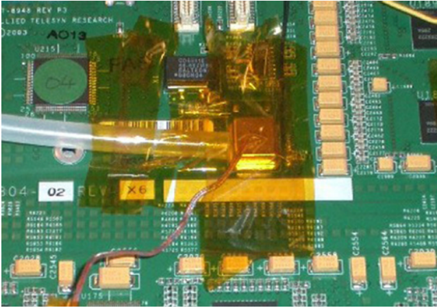
Figure A2.1 Freeze spray is applied to a suspect component
