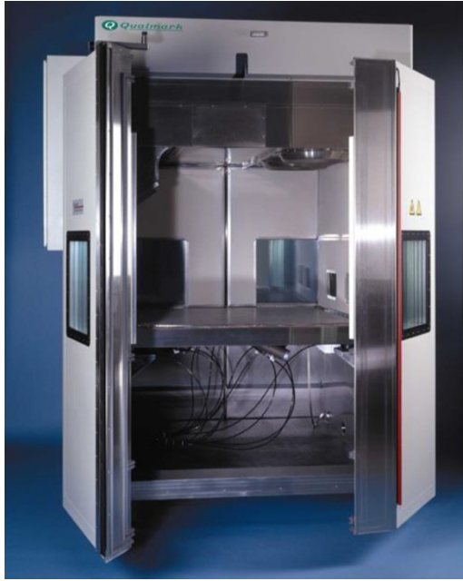
Figure 6.5 Typical HALT chamber. Source: QualMark 2015. Reproduced with permission of QualMark Corporation
