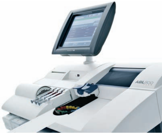
FIGURE 14.5. ABL800 FLEX blood gas analyzer. (Reprinted with permission from Radiometer America Inc., Westlake, OH.)
