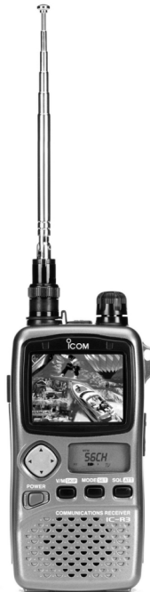
Figure 5.14 A high quality communications receiver that uses the superhet principle (courtesy Icom UK)
