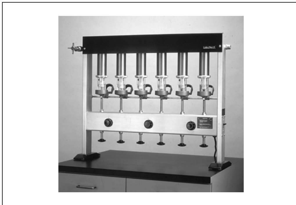
Figure D1.1.2 Goldfish lipid extraction unit (Courtesy of Labconco Corporation, Kansas City, MO). A single beaker is used as the solvent chamber. Samples are placed between a boiling solvent and a cold surface. The solvent vaporizes, condenses on the cold surface, and washes down through the samples into the boiling solvent below.
