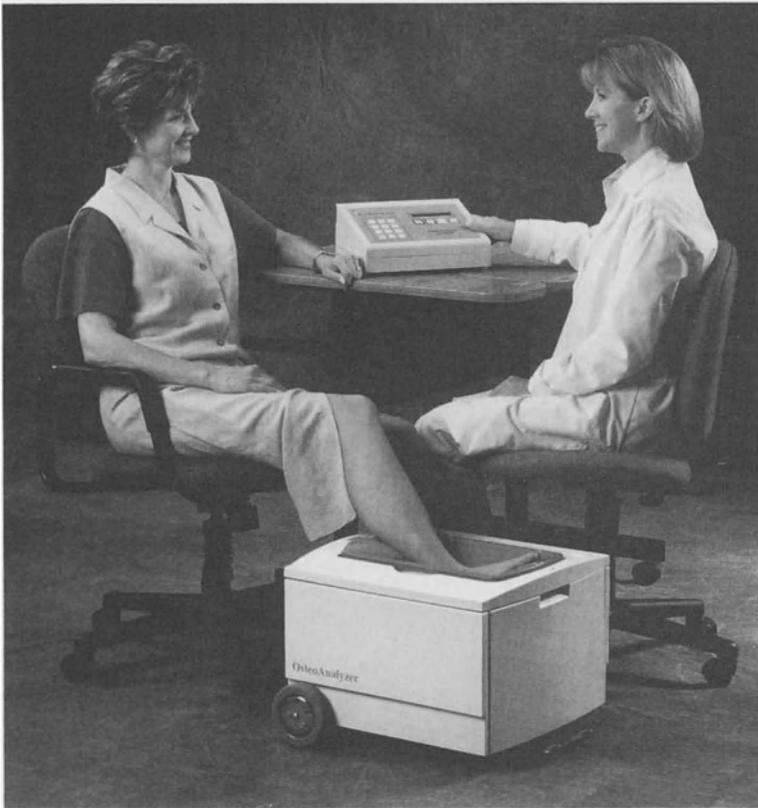
**Fig. 1-19.** The Norland Analyzer, a portable SXA device for measurement of bone density in the os calcis. Photo courtesy of Norland Medical Systems.
