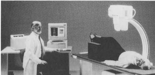
**Fig. 1-13.** The Lunar Expert, a fan-array DXA device. Photo courtesy of Lunar Corp.
