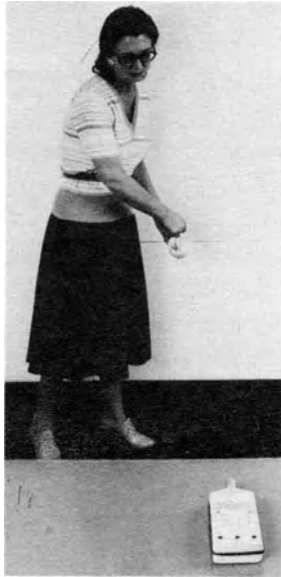
Figure 10 Checking level of sound used with a Dawe sound level meter. The cup and spoon were 1 m away from and level with the meter
