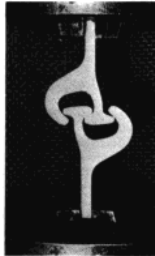
Fig. 6.27. Flat pile sections (a) modern sections with high strength interlocks, and (b) alternative sections previously available showing single point (left) and three-point contact (right) at interlock (courtesy of Arbed)
