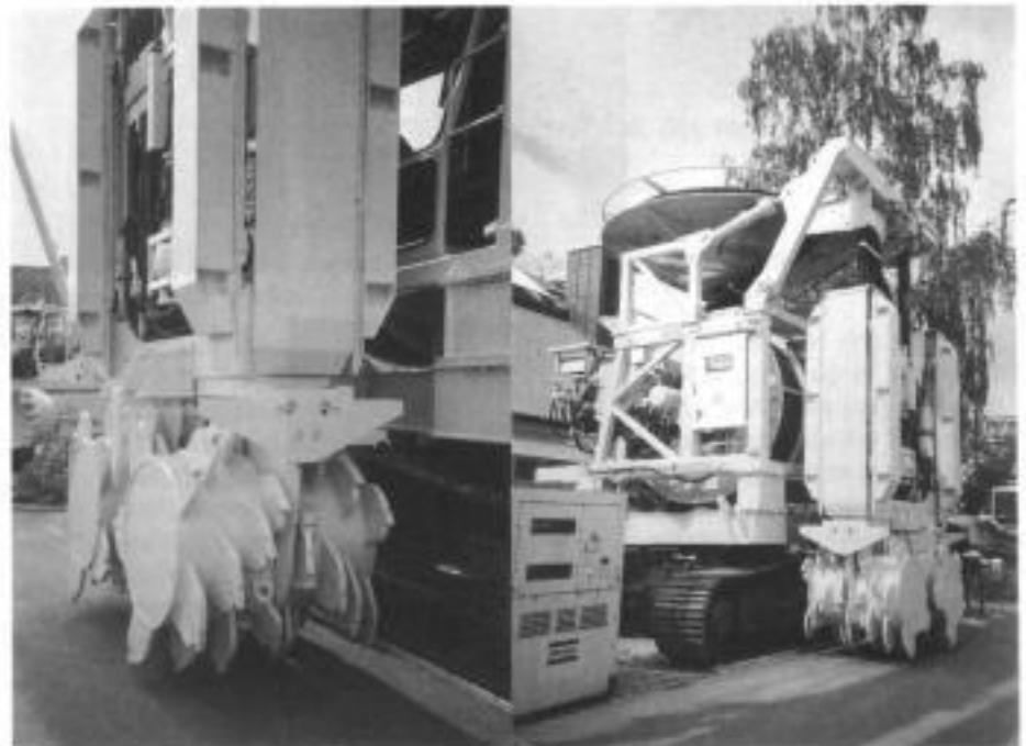
Fig. 8.20. Bauer City Cutter rig: use of alignment device on small base machine to improve manoeuvrability in limited space
