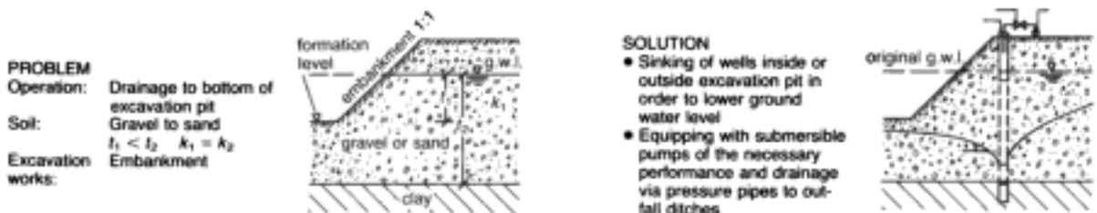
Fig. 2.2. Groundwater control applied to a battered excavation
