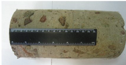
FIG. 3. Core sample drilled out from jet-grouting column in clay.
