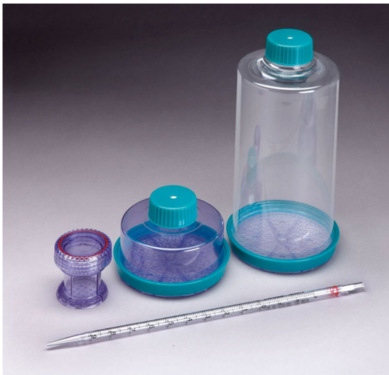
Fig. 6.5 Gas permeable flasks that have been used for T cell culture. These flasks have a gas permeable member at the bottom (G-Rex, Wilson Wolf Manufacturing, New Brighton, MN, USA). Three different size flasks are shown. The smallest flask, G-Rex10, has a gas permeable membrane of 10 cm 2 and a capacity of 40 mL. The middle and largest size flasks both have membranes of 100 cm 2 ; the middle flask, G-Rex100, has a capacity of 500 mL and the largest flask, G-Rex100L, has a capacity of 2000 mL
