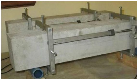
Fig. 4 Drying shrinkage test specimens [8]
