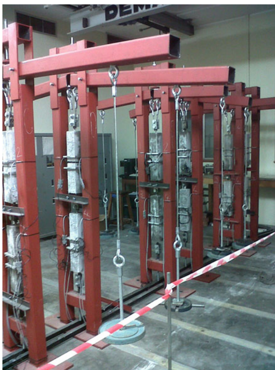
Fig. 3 Tensile creep frames showing specimens under sustained loadings [8]
