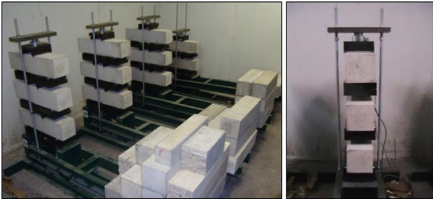
Fig. 2 General view of creep test specimens (overview -left- and column detail -right-)
