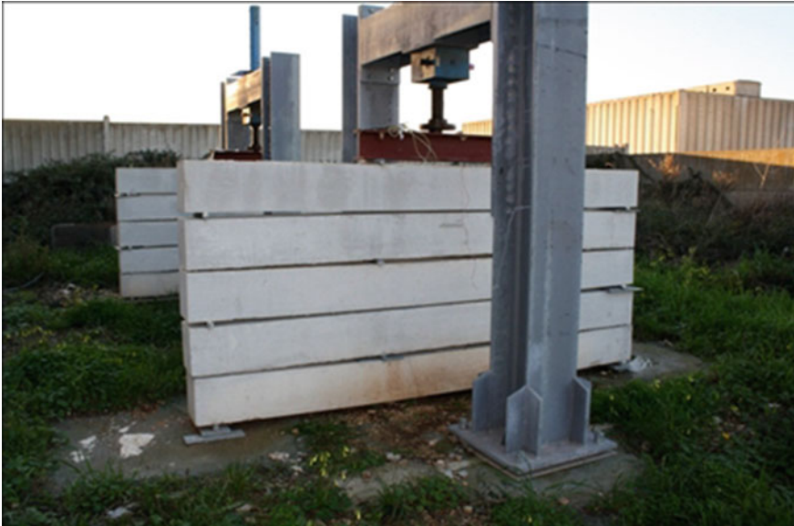
Fig. 1 The two exposure loading frames
