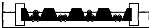
Figure 4. A schematic of the culture wafer suspended in medium with tube supports
