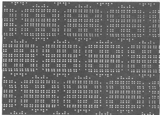
Figure 2: A micrograph of the Design I cell culture wafer. The etched holes on the filter membrane are 3\ \mu\text{m} in diameter.
