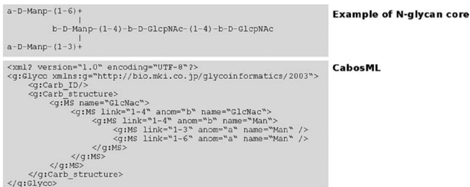
Figure 3.13 CabosML encoding of the N-glycan core. Topologies are reflected by the parent–child relationships of the element g:MS .
