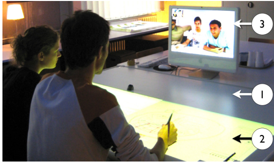
Fig. 1. The Collaborative Digital Studio: (1) Projected work surface, manipulated by a physical stylus, (2) SketSha annotation software, (3) Video-conference device
